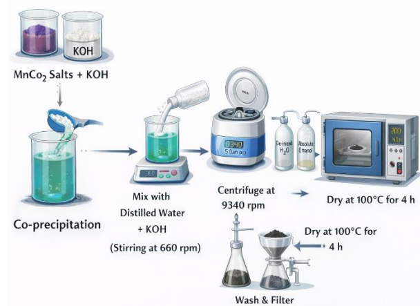
Fig. 1 Synthesis schematic of the \text{MnCo}_2\text{O}_4 prepared via co-precipitation method.
